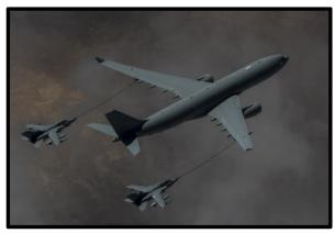
**Voyager** is the RAF's sole air-to-air refuelling (AAR) tanker and also operates as a strategic air transport. Fuel offloaded during AAR is taken from the aircraft's standard wing and fuselage tanks, leaving the cabin free for up to 291 personnel and the hold available for freight.
